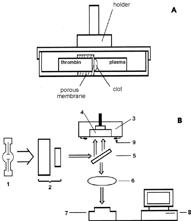
Fig. 1. Scheme of the laboratory set-up. (A) Scheme of the polystyrene chamber. (B) Scheme of the laboratory set-up: 1, mercury lamp; 2, light-blocking filters; 3, thermostat; 4, polystyrene chamber; 5, interference mirror; 6, optic focusing system; 7, CCD camera; 8, computer; and 9, diodes.
