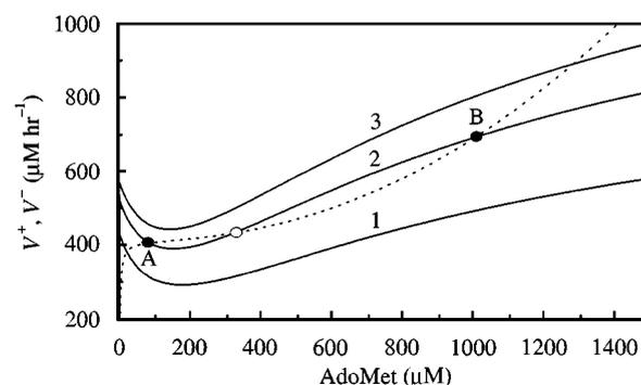
FIG. 4. The total rates of AdoMet production ( $V^+$ , —) and consumption ( $V^-$ , - -) as a function of AdoMet concentration.  $V^+$  is shown at three different methionine concentrations: 1 is at 42.5  $\mu\text{M}$ , 2 is at 52.5  $\mu\text{M}$ , and 3 is at 57.5  $\mu\text{M}$ . (●) indicates stable steady states with low (A) and high (B) AdoMet concentrations; (○) indicates an unstable steady state.
