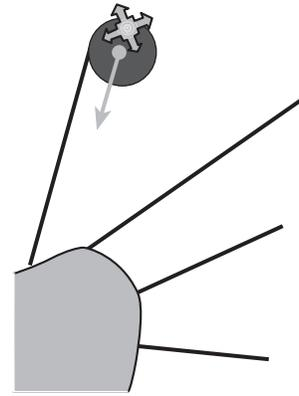
**Fig. 1.** Schematic representation of experiment. One microtubule is connected with a bead used for the experiment. When the depolymerization wave approaches the bead, it is affected by the force shown by the arrow. This results in the movement of the bead relative to the trap center marked by the cross.
