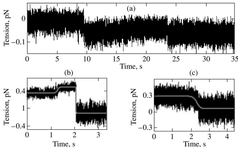
**Fig. 2.** Examples of signals obtained from the quadrant detector: (a) Both events occurred after the addition of calcium and before complete liberation of the bead; (b) a signal which demonstrates the force development; (c) an experiment without any force, with relaxation to the free state. The solid curve shows approximation by the smooth function.
