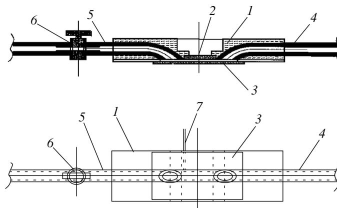
**Fig. 1.** A schematic representation of a flow cell. 1—Flow cell framework; 2—glass; 3—biochip; 4—inlet pipe; 5—outlet pipe; 6—valve; 7—additional capillary tube. Total channel length is 33 mm, width, 6 mm, and depth, 1.3 mm. Internal inlet and outlet pipe diameter is 3 mm. The distance between the hole edges is 21 mm.
